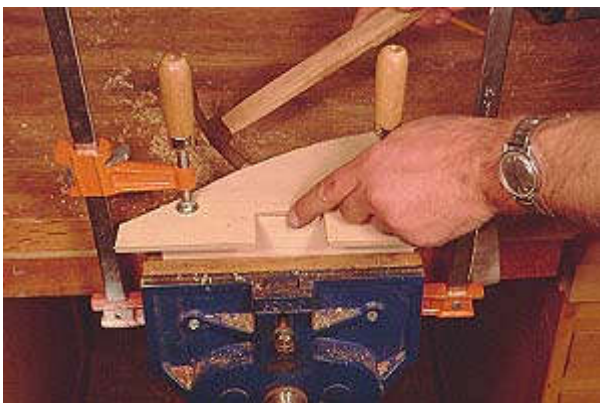
Photo 6- Locating the hinge template on its fence. Clamp the two together, carefully measure how far the back of the 'U' is from the fence, tap with a hammer to adjust, then screw or nail the template to the fence.
