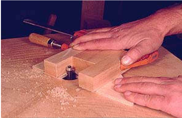
Photo 3- Flush trim the plywood to the shape of the primary template on the router table using a bearing guided flush trim bit.
